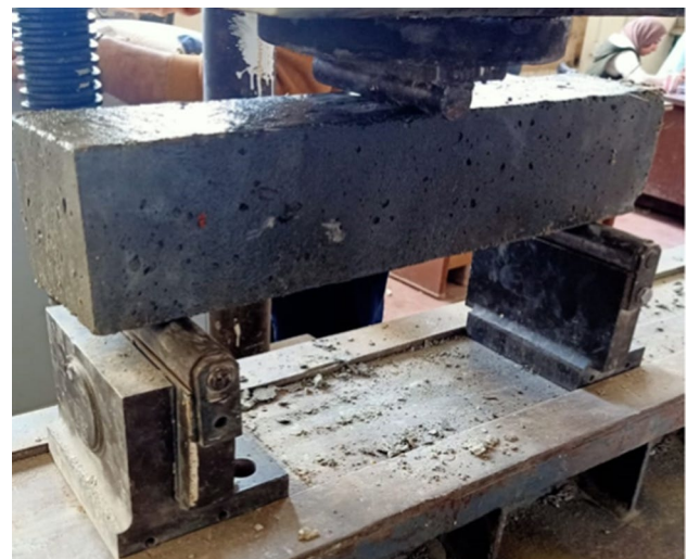
Fig. 3 Flexural test setup
