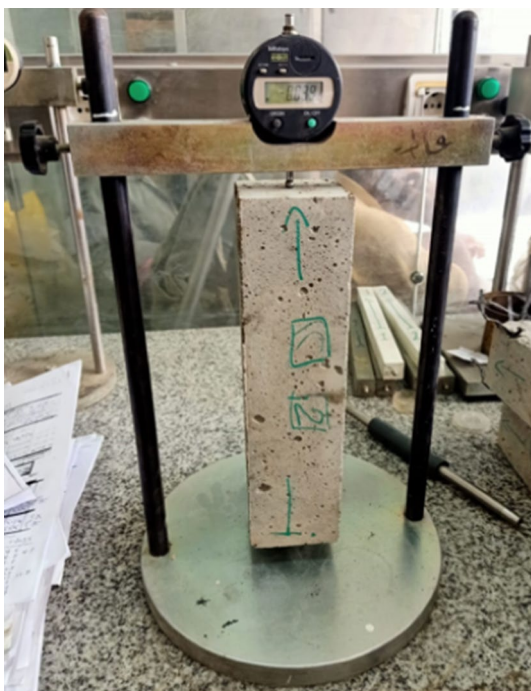
Fig. 4 Drying shrinkage test setup
