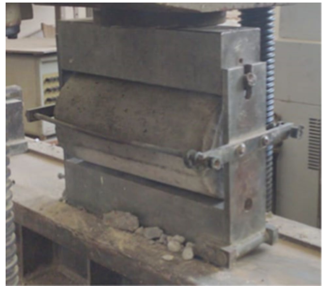
Fig. 2 Splitting tensile test setup
