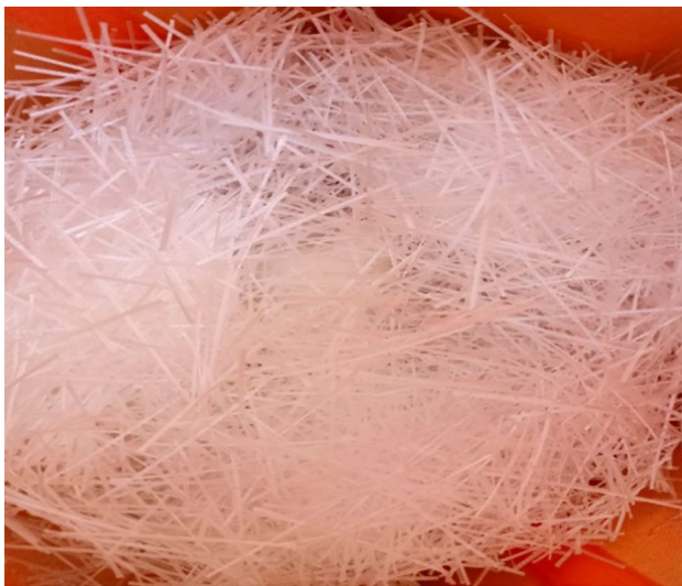
Fig. 1 Structural macro-synthetic polypropylene fibers
